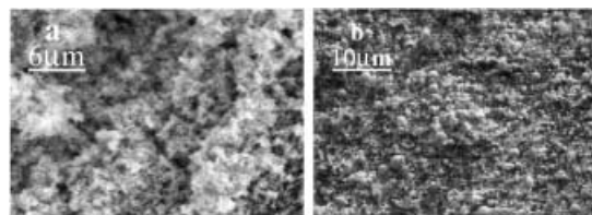
Figure 6. SEM images that show the typical morphology of MoCO crystalline products obtained at 80°C with the argon flow rate at about 50 sccm.
